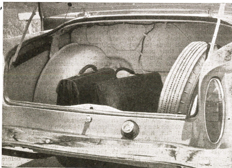
Luggage space is generous. Spare wheel and tools are located on the right hand side of the boot, leaving the rest of the space free.
