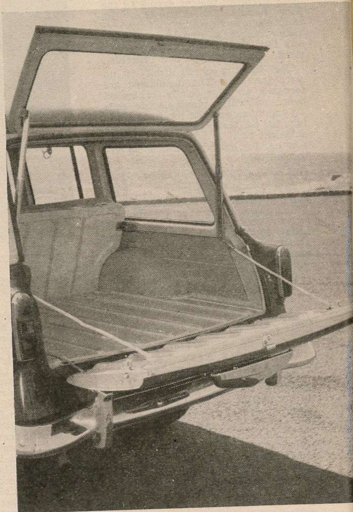
Tailgate and transom both open wide for easy loading. All fastenings are sturdy and rattleproof — but no provision is made for locking top portion with tailgate in down position.
