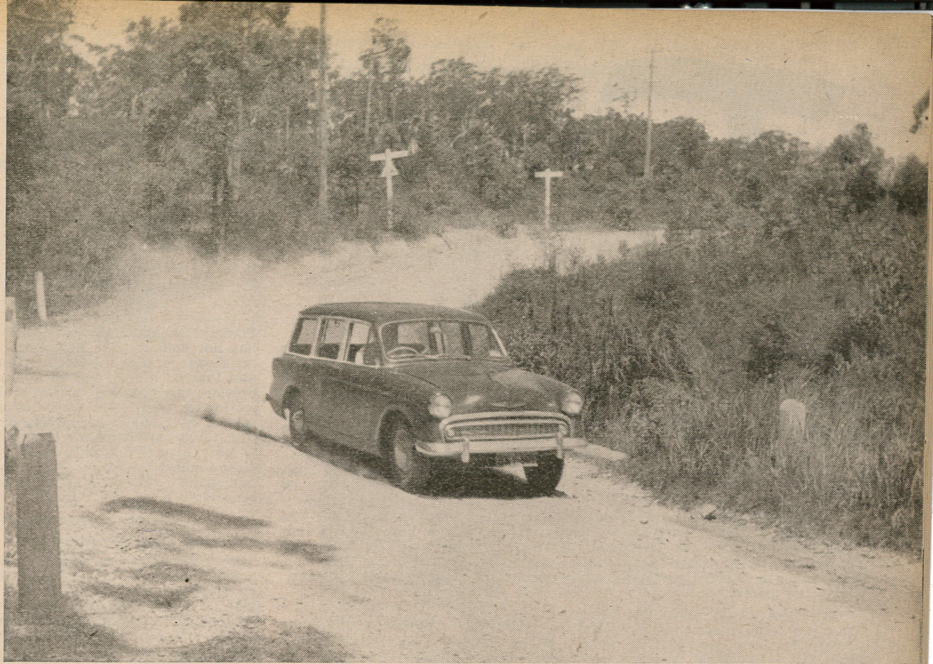
Tremendous stability on gravel came as a major surprise. Tail slides can be corrected with a flick of the wheel, while the suspension takes all that is coming—and then some.
